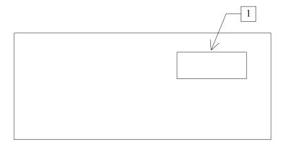
AC POWER INPUT. A three-pronged recessed male connector is provided on the back panel for AC power connection to the instrument. Also contained in this assembly is a slow-blow fuse and a removable card that can be removed and repositioned to switch between 120V AC in and 240V AC in.
